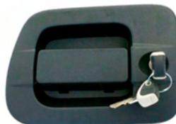
MAÇANETA EXTERNA COM CHAVE IVECO STRALIS/TECTOR LE
