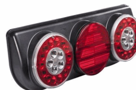
COD:1109900 LANTERNA LED FACCHINI BRASPOINT IV 24V LD
